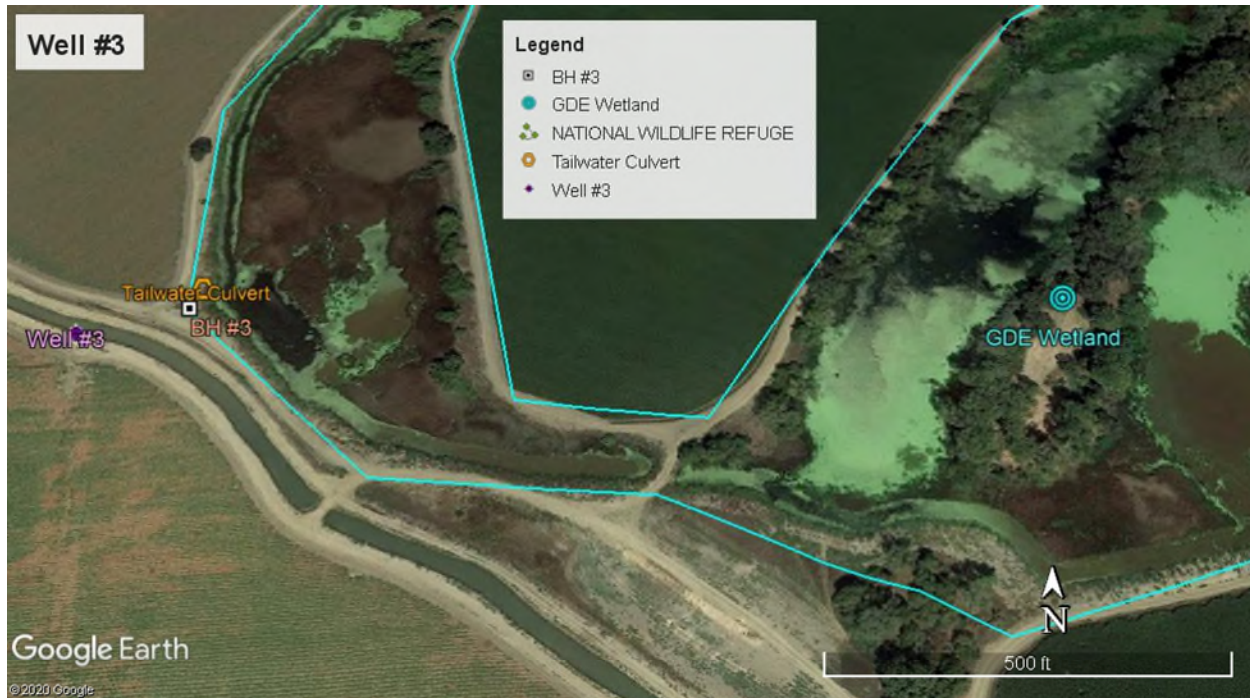
Figure 5: Detail of Well #3 Proposed Location in relation to GDE areas. Location of proposed well was moved approximately 200 feet away from edge of wetland to reduce species impacts on birds, amphibians, and reptiles.
